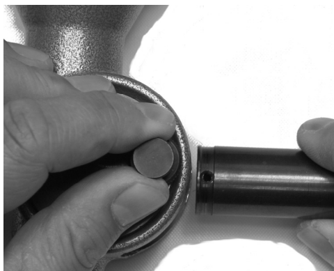
Aligning locking pin hole on metering assembly
