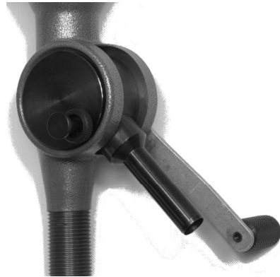
Powder hopper “drain” position
