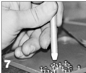
The primers will now be oriented anvil side down for easy pick-up with the appropriate size priming tube assembly. See photo 7.
