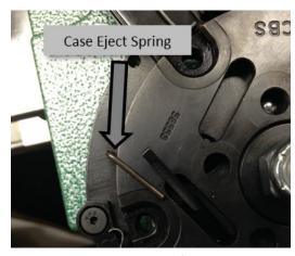
**Photo 18 Top View of Case Eject**
