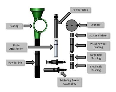
**Diagram F. POWDER MEASURE ASSEMBLY COMPONENTS**
