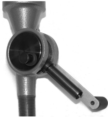
Powder hopper “drain” position
