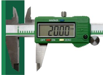
Differential method measurement (Application of zero setting)
