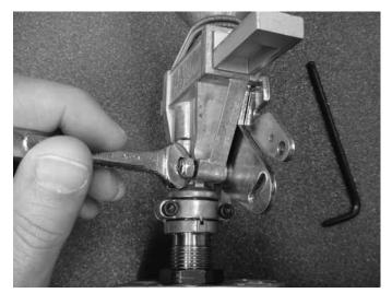
Photo 2. PM Bellcrank Locknut
