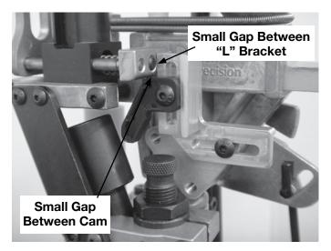
Next, reinstall the PM Failsafe Rod to the Bellcrank Brackets (consult your Powder Measure Manual for more information). Place a properly sized/ trimmed case at the powder drop station and fully lower the Press Handle. The Cam on the PM Assembly should engage the Push Bar and drop a bullet into the Seat Die Assembly. Ensure that the Cam does not contact any other components throughout its range of motion.
