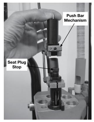
Manually squeeze the Bullet Feeder's Push Bar Mechanism, allowing the bullet to drop into the Seat Die Body (Photo 11). Visually check to ensure the bullet has dropped down inside the Guide bushing under the Seat Plug. If it did not, the Seat Plug needs to be positioned higher to allow the bullet to drop. See Adjustment section for more information.
