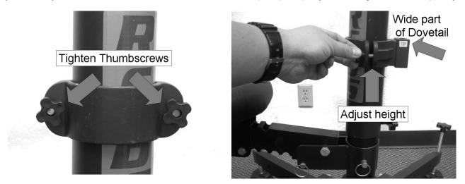
Attach the Tray Top assembly to the Clamp. The dovetail features a 'bayonet' type mount, slide the bottom half of the Tray Mounting Brace into the Mount Receiver and press downward. (See photo)
