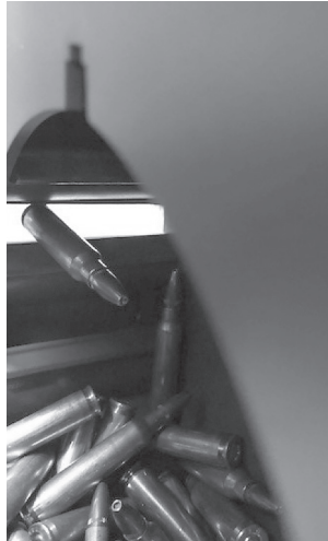
Hopper Jam ( view from hopper door area )
