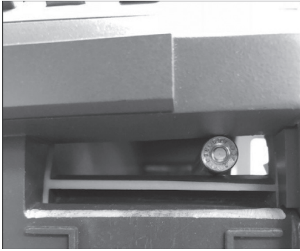
Hopper Jam ( side panel removed )
