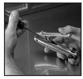
Photo 7: Centering Internal Linkage
