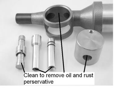
Install the Locking Pin assembly into the single threaded through hole on the side of the Measuring Cylinder and tighten. Carefully insert the assembly into the main casting, this is a precise fit, do not force the cylinder into the casting. Insert screws through the handle and attach to the measuring cylinder on the opposite side of the Locking Pin. The Powder Measure can be set up for right or left handed use depending on which way you slide in the assembly.
