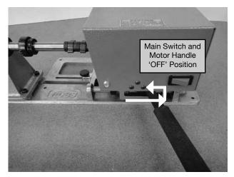
Photo 9. Motor Handle Locked in OFF Position
