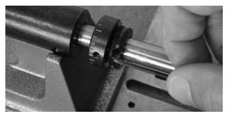
Photo 17. Coarse Adjustment Bushing
