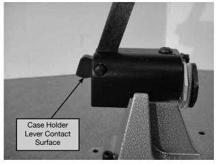
Photo 21. Lubricate Case Holder Lever
