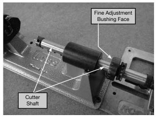
Photo 20. Lubricate Cutter Shaft and Fine Adjustment Bushing Face
