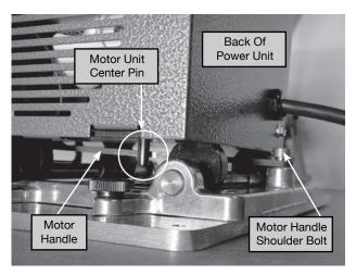
Photo 23. Lubricate Contact Surface of Motor Unit Center Pin (on Bottom of Motor) and Motor Handle
