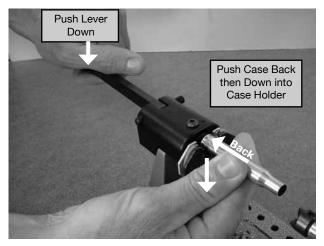
Photo 11. Inserting Case into Universal Holder
