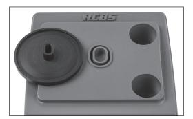
Photo 4: Align feature on platen and load cell
