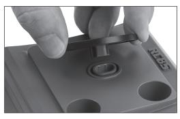
Photo 5: Insert platen into load cell pocket
